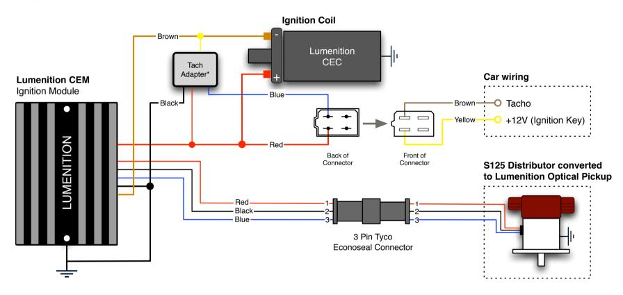
This setup is a replacement for a Dinoplex C or AEC 103A, The setup based on a Lumenition Optronic Performance constant energy inductive ignition (CEM) combined with an optical pickup (CET150) and coil (CEC). The Lumenition Optronic Performance optical pickup CET150 requires an adaption kit containing a trigger wheel (chopper) such as the F425 or F009.
